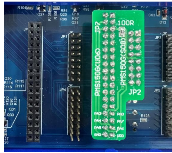
Fig. 15: JP2 Physical connection diagram
